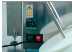
Electronic check of weld temperature
